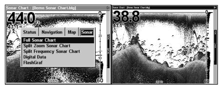
Pages Menu, showing sonar chart display option commands (left). Sonar Page in full sonar chart display mode (right).
